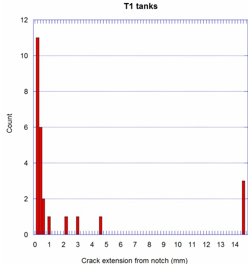
3 tanks, 8,000-15,000 cycles per vessel
