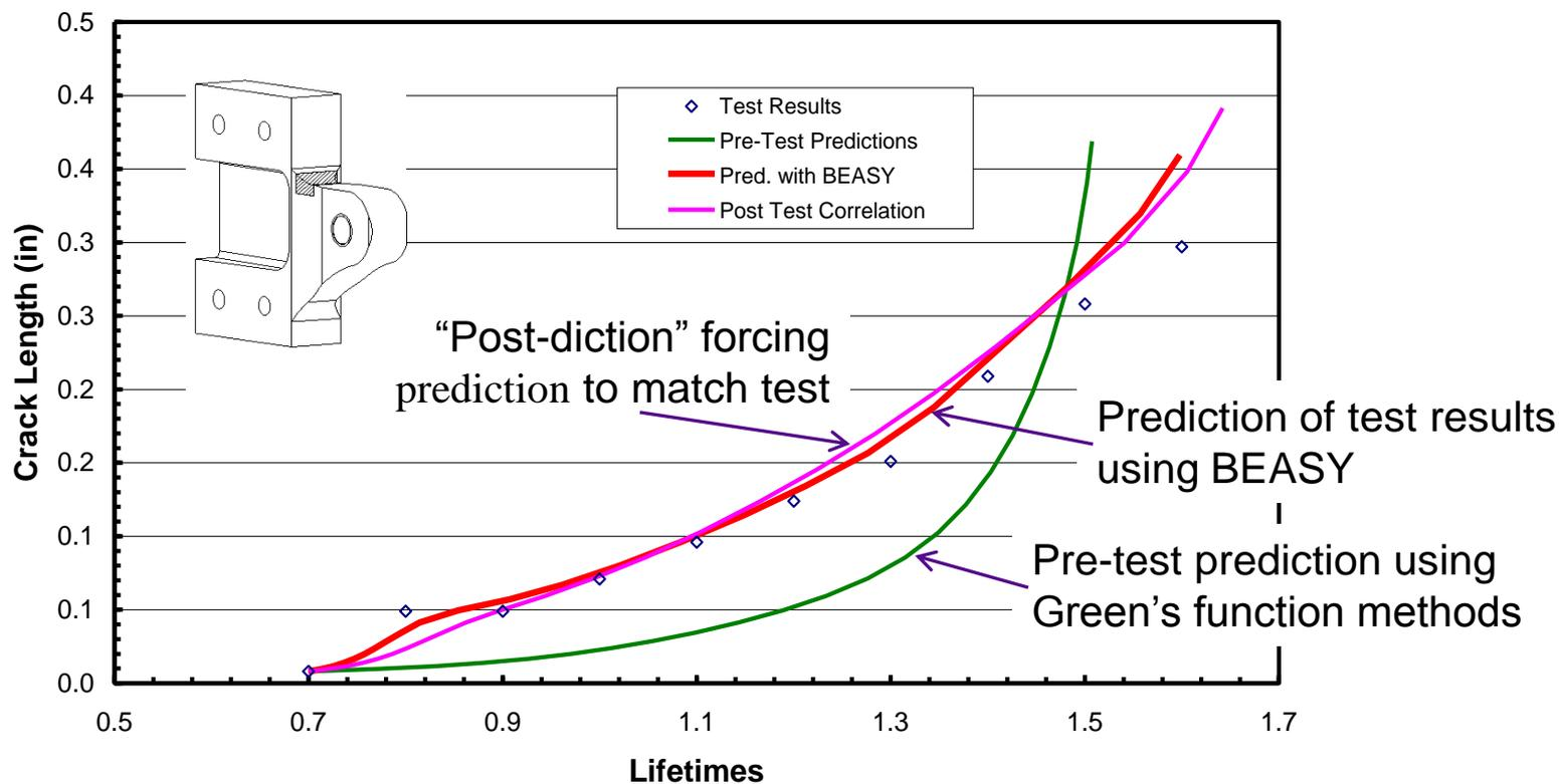
Crack growth predictions using stress intensity factors from the boundary element analysis match test results
