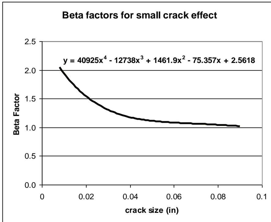
For Ti-6Al-4V Beta Annealed, 2.54 mm (0.1”) is approximately 2 to 3 grain diameters. A range where microstructural features can strongly influence crack growth.
