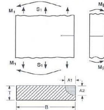
Cross section of fracture surface shows greater complexity than provided by simplified stress intensity solution
