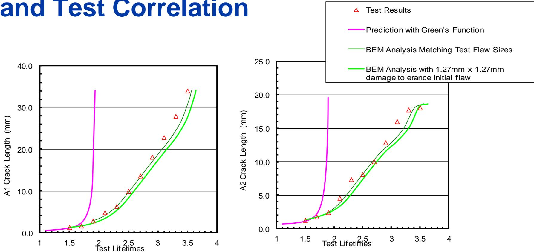
Analytical results are from crack growth analysis with different stress intensity solutions:
