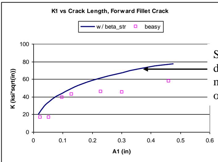
Stress intensity factors derived using current method higher than those obtained from BEASY
