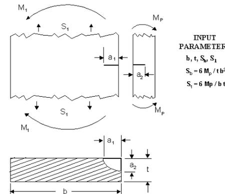
CASE 120. Single Corner-to-Corner Edge Crack,
