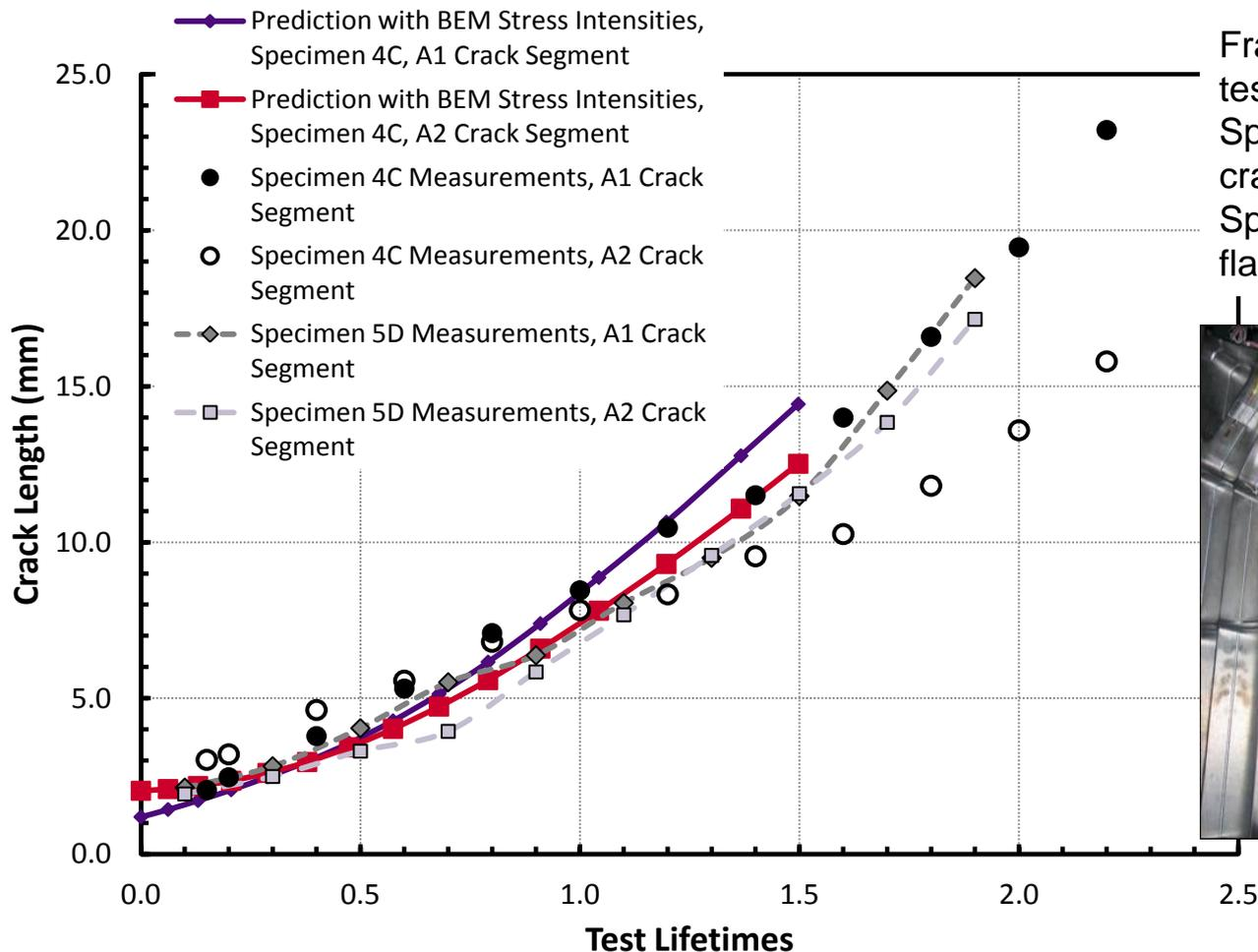
Frame 4 component crack growth test results.
