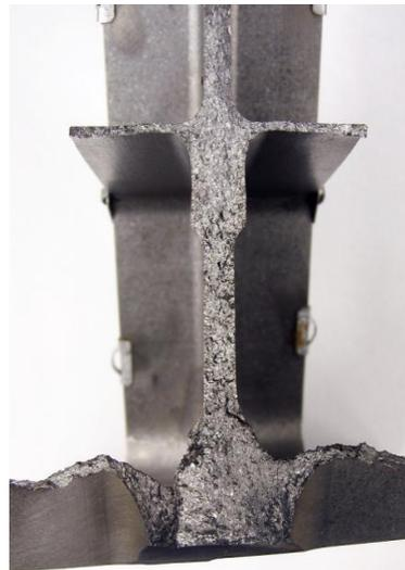
Crack origins at lower corners
