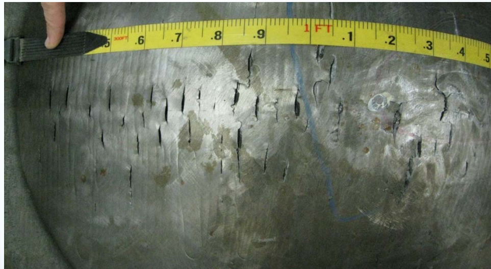
EB Specimen slow-1 (HI~1.3 kJ/mm)
